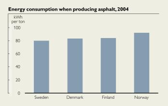
Energy consumption required for the production of one ton of asphalt ranges from 80 to 92 kWh.Variations are due largely to weather conditions.
